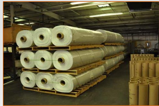
Master rolls of plastic ready to be cut to size
