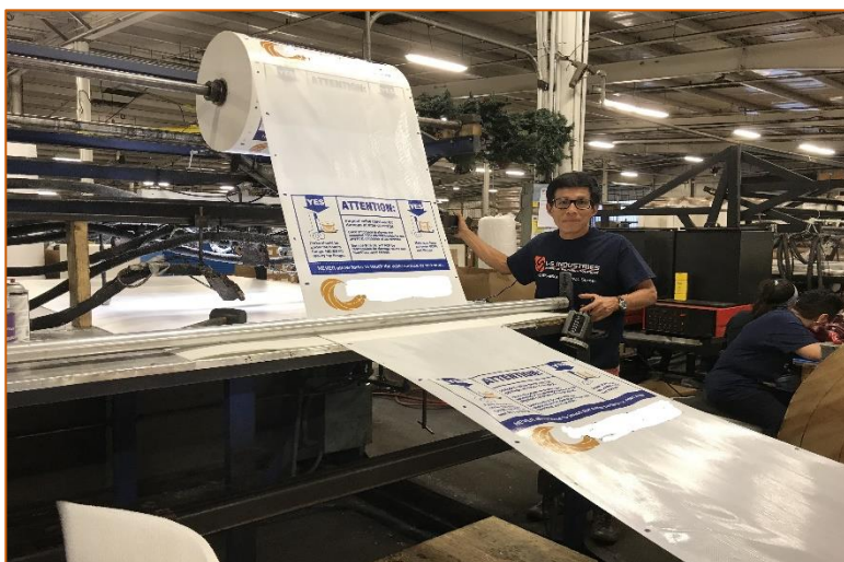
Laminating rolled and sheeted materials
