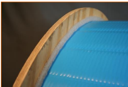
Foam overlap up against the flange
