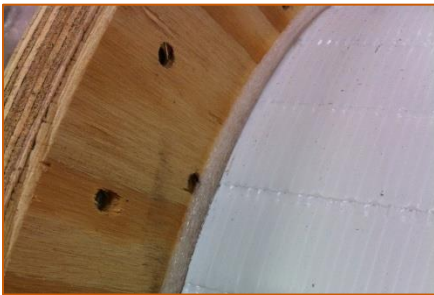
Foam overlap creates a tight seal
