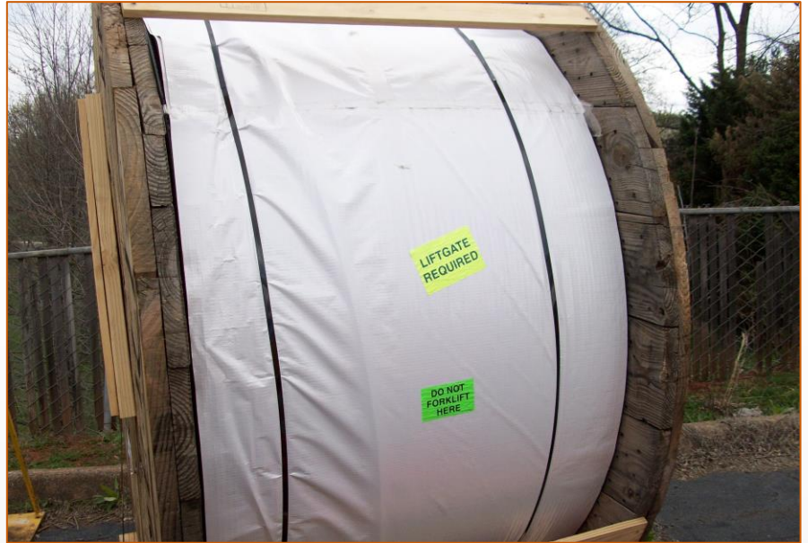
Thermal Wrap keeps heat away from the product
