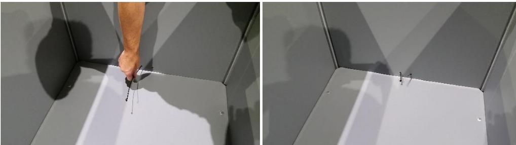
*NOTE: Only heavy-duty 0.76"+ thick cable ties are to be used. Standard zip ties can break easily when the bin is loaded down.*
