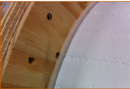
Foam overlap creates a tight seal
