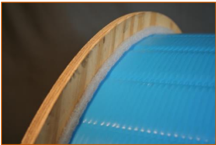
Foam overlap up against the flange
